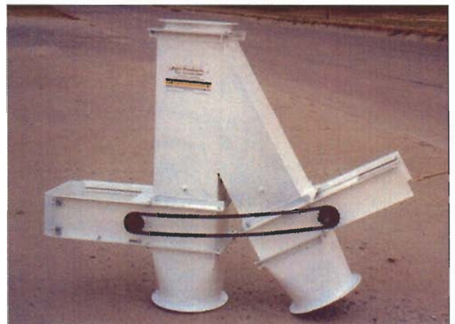
Rack and pinion diversion valve with "timed" chain drive to open and close gates
