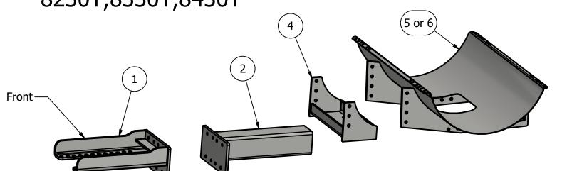
**Bolt List** QTY Description Placement 3/4 x 4 1/2" Bolts Brackets to Hardbar on tractor 3/4 x 2 1/2 Bolts **Tubes to Brackets** 3/4 x 2 1/2 Bolts Conversion to Saddle 3/4 x 7 x 9 U-bolts Conv. to Tube 3/4" Lockwashers 36 3/4" Nuts 60 20 mm Hardened Flatwashers **Brackets to Tractor** 1 1/2 OD x 1 IN Bushing x 3/4 Spacer between bracket & Hardbar Nylon Straps Tank to Saddle
